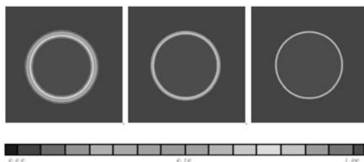
(a) The contour of density distribution for different lattices (from left, lattice 50x50, 100x100, 200x200)
